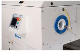
A temperature sensor mounted at the exit of the sterilizer monitors the temperature of each end as it exits. The system is controlled by a microprocessor, which automatically adjusts the power level of the sterilizer to produce ends at the operator pre-set temperature.
