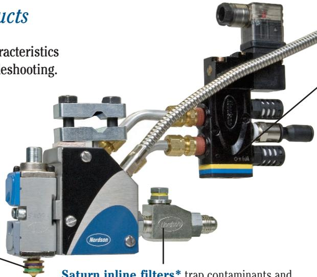
**Saturn solenoid valves\*\*** optimize hot melt dispensing gun performance with high air-flow capacity for better cutoff and high-temperature seals for longer life. Rings identify voltage and air flow (Cv value). Designed specifically for hot melt adhesive dispensing, valves are available in 3-way and 4-way air-open/spring close and air-open/air-close designs.
