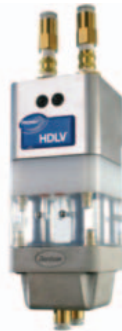
The HDLV powder feed pump transports precise amounts of powder from a feed source to a powder spray gun. The pump consists of two halves that function identically while isolating the suction and dispensing processes. The halves alternately draw powder in and dispense powder out of the pump.
