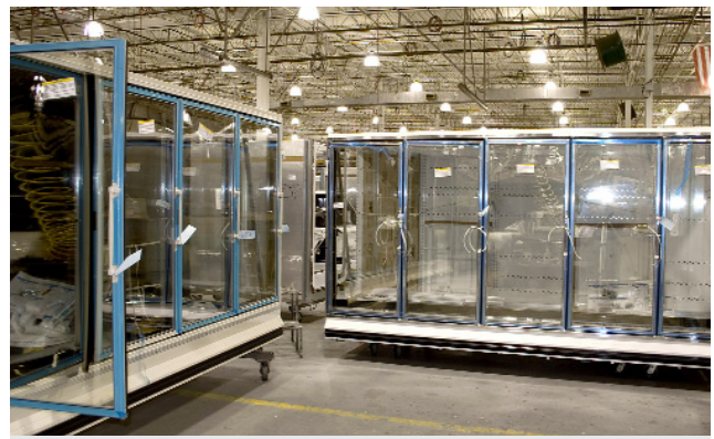
Each refrigeration display case is manufactured and powder coated based on a custom order, which means 90 to 100 color changes on average during each two-shift day.
