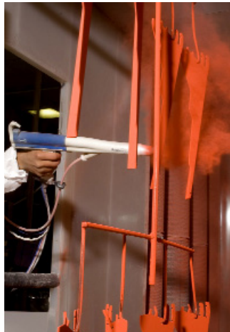
Use of Nordson Prodigy® HDLV® technology has led to a decrease in color change time by as much as 70 percent. Non-reclaim color changes that previously took from 1.5 to 3 minutes now take about 30 seconds.
