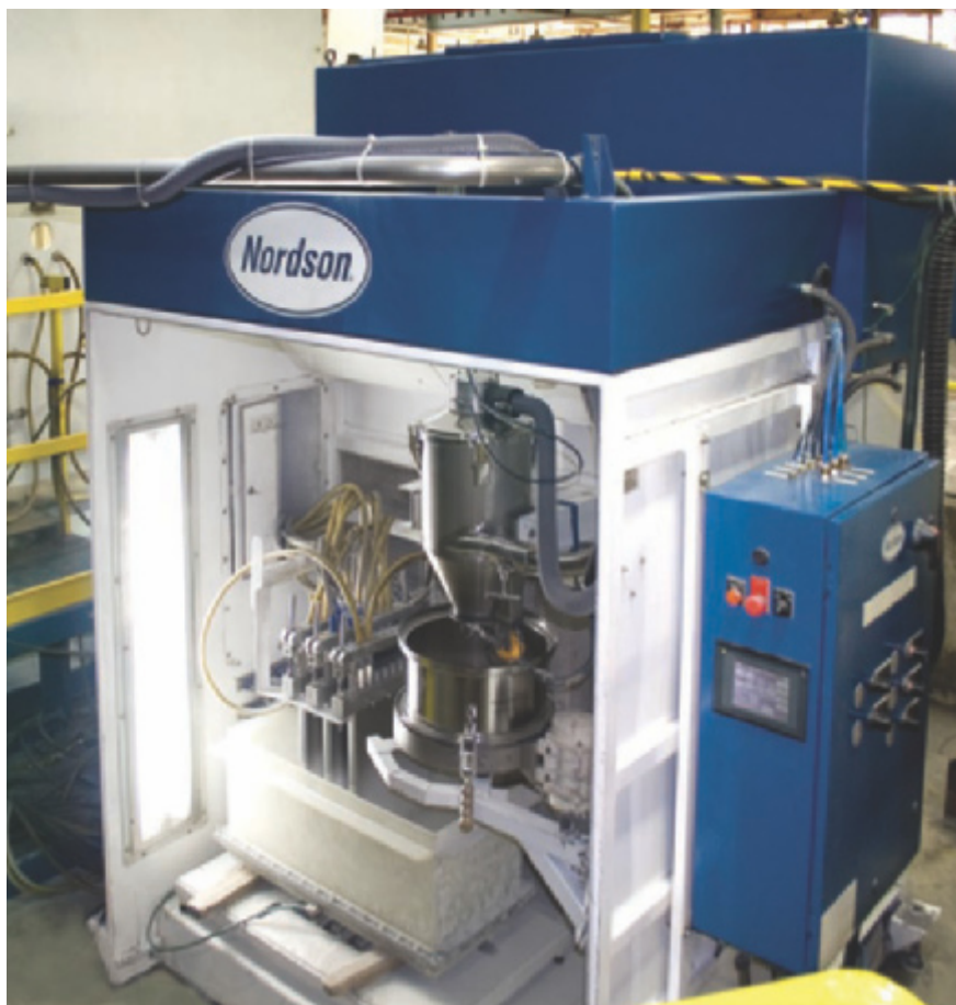
A powder feed system supplies the spray guns and automatically recovers, sieves, and recycles powder overspray for improved material use and reduced loss.
