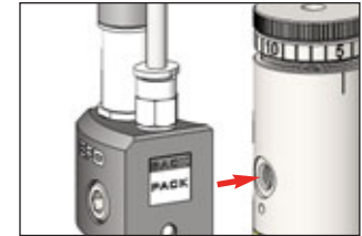
Step 2. Secure Backpack actuator pod to air cylinder inlet opening
