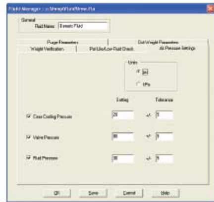
Electro-pneumatic regulators control valve, fluid, and cooling/coax pressures. Pressure values are set in FmXP software and monitored directly from the computer screen. Gauges are removed from the front panel.
