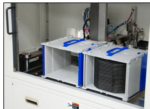
Unprocessed film-frame wafers are pulled from one cassette and returned to a second cassette once processed
