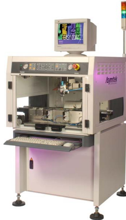
Automated Coating Platform
