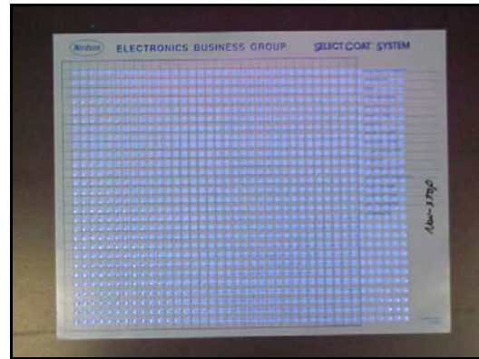
1120 Dot Grid Jetted with 100% Solid Silicone. 4mm Dot Diameter.
