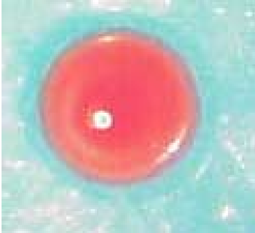
Figure 10. SMA dot jetted onto an organic substrate.
