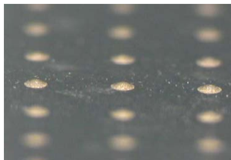
Figure 3. MA-2 Silver Dots on Glass Slide, Side View
