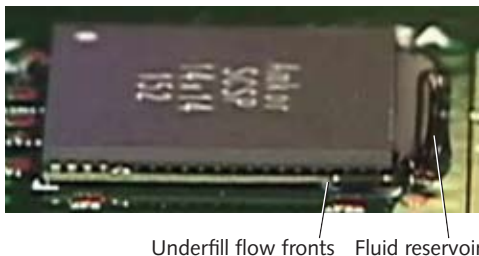
FIGURE 5. Simultaneous underfill of both PoP layers.
