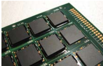
FIGURE 3. RF shield providing access for underfill.
