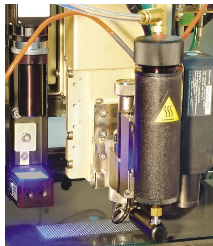
Figure 2. Jet with hot-wax feed system for use in the life sciences and hard disk drive industries.
