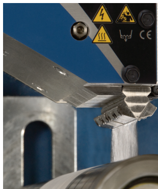
Patented porting of process air, (both parallel and angled) to the adhesive output produces random, continuous filaments with excellent cutoff.
