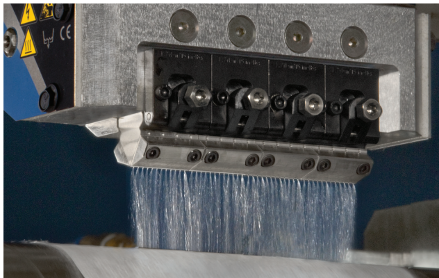
A greater nozzle-to-substrate distance decreases exposure to airborne contaminants that can compromise performance.
