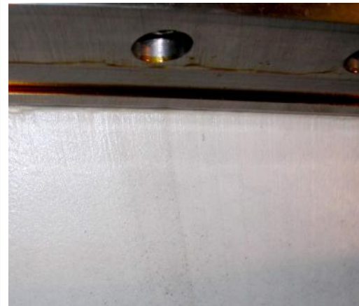
Slot Coating of Foamed Adhesive
