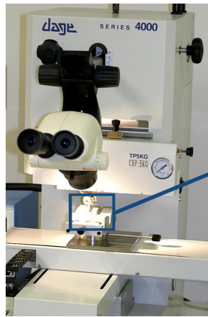
Nordson DAGE 4000 bond tester performing a cold bump pull test
