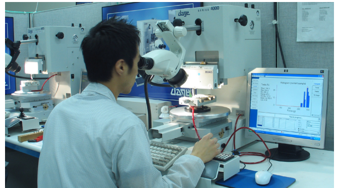
Nordson DAGE 4000 bond tester performing a wire shear test
