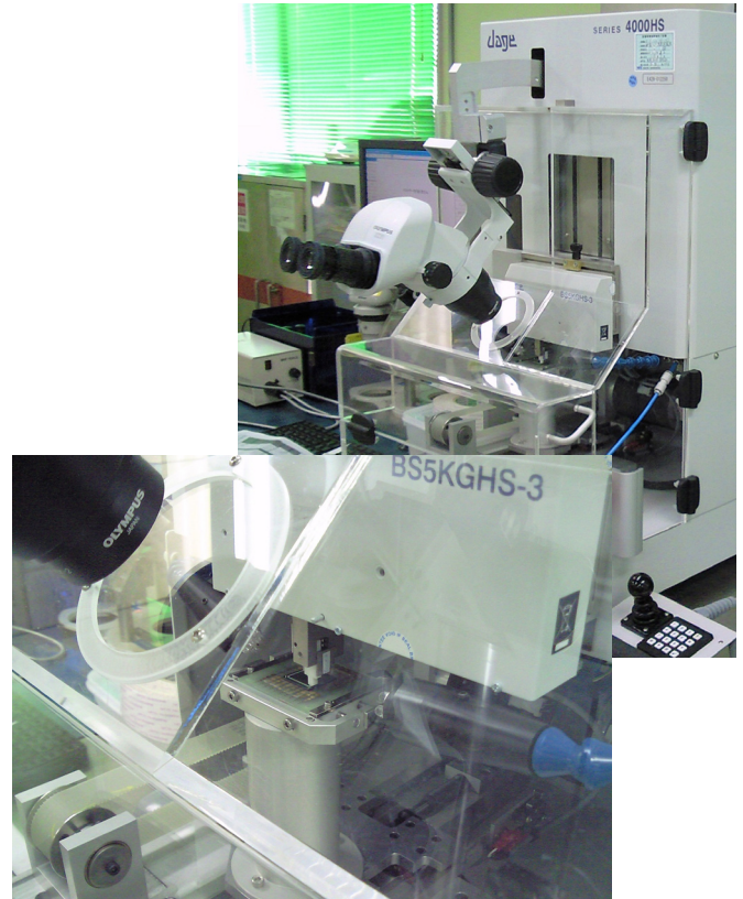
Nordson DAGE 4000HS bond tester performing impact shear test
