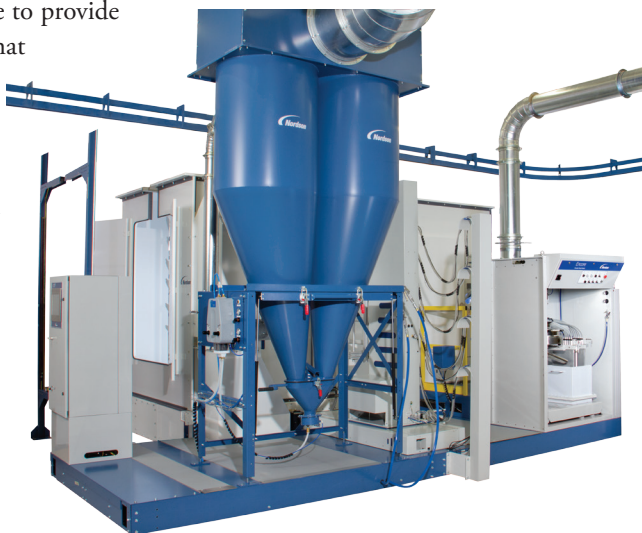
The Colormax® quick color change system is capable of color change times of seven minutes or less.
