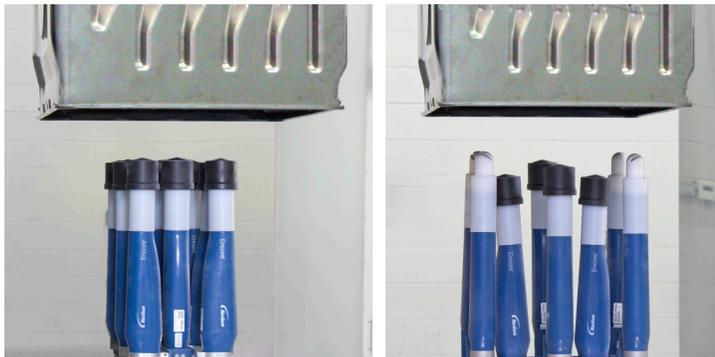
Encore PE-HD multi-gun arrangements for coating cavities
