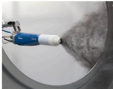
Encore PE-HD Automatic Bar-Mount Gun with Flat Spray PE Nozzle
