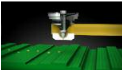
Dispensing on an uneven substrate
