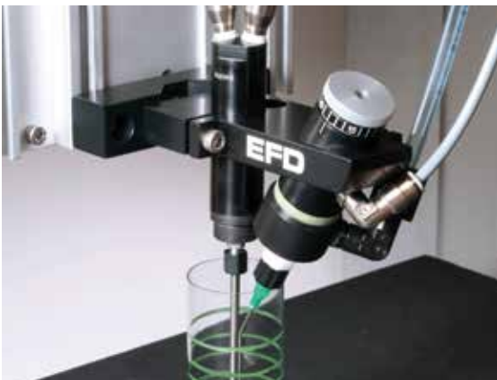
Radial spinner valve coating internal walls
