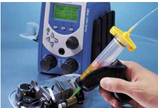
Ultimus dispensers feature time adjustment \geq 0.001 seconds for exceptional control.
