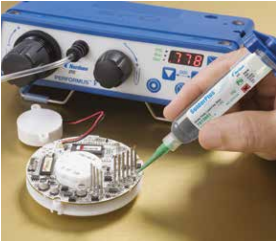
Performus V provides excellent process control in solder applications.
