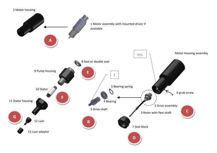
A. Slide the motor assembly (1) into the motor housing (2), position it and tighten them together with 4 x hex screws M3 x 8 (19).
