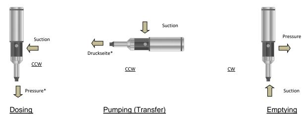
INFINITI pumps in general can be used in two directions: Clockwise or Counter Clockwise. Furthermore, the position/angle of the pump almost does not have any effect on the pumping or dosing result. Only in some cases, the suction performance can be influenced by it.
