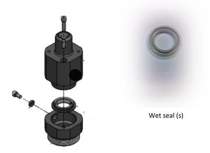
The rotor-drive-assembly is made of 1 piece only and cannot be dismantled. Please only use inert lubricants for assembly. Generally, they are not needed and can leave unwished residue. Never use silicone based lubricants for automotive applications because they are forbidden.
