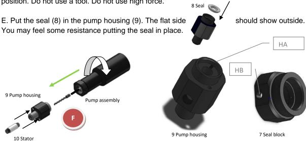
F. Put on the stator (10) and tighten it by hand only. Gently screw the pump assembly into the stator and make sure, that both wholes (HA, HB) are positioned over each other. Connect them with the 2 hex screws M3 x 10 (20). Please check 4.1.1.1 on the over next page!
