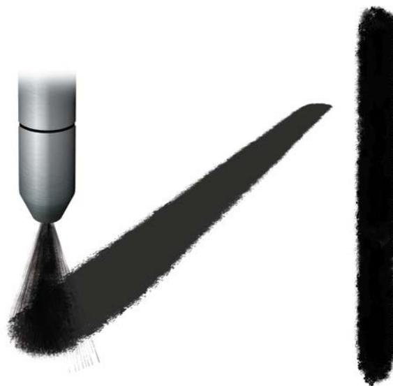
**Figure 3.** Atomized spray coater.
