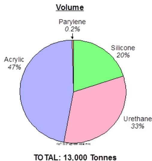
**Figure 2.** Conformal Coating Materials 2013. Courtesy of Prismark Partners, LLC.
