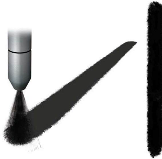
Figure 3. Atomized spray coater. Applicator tip with spray pattern (left), top view of spray pattern (right).
